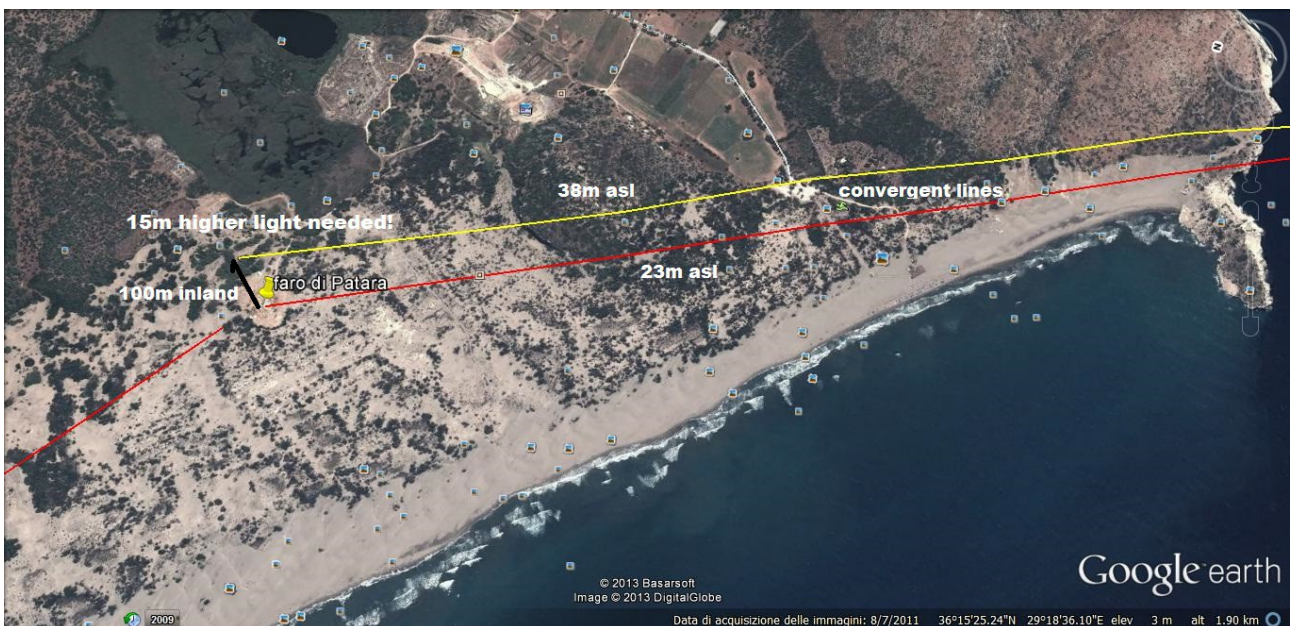
One hundred metres inland, and it doesn't simply work, anymore. Unless the tower is fifteen metres higher.
